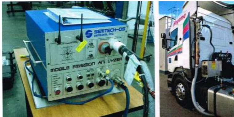
Figure 4. SEMTECH DS (a) and a flowmeter to measure the mass flow of exhaust gases installed in exhaust system of the test vehicle (b)
